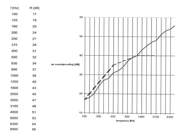
f -frequency [Hz] R 1/3 octave -air soundproofing index [dB];  $R_w(C,C_{tr}) = 36$  (-1; -6) dB
